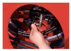
It is an advantage to boom integrity to pre-load these rams periodically via the boom control levers.
