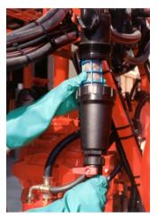
This extra fine mesh filter is fitted directly before the boom manifold and is particularly useful for low volume work where crystallising chemical presents a problem.
