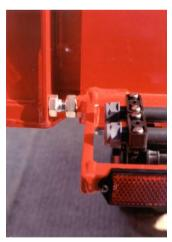
Screw stops are situated where the booms fold and these should be regularly checked for tightness and boom alignment.
