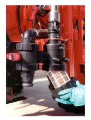
A large capacity suction filter is fitted on the left-hand side of the machine behind the wheels. The 30-mesh element should be cleaned frequently to eliminate pump cavitation and loss of spraying pressure. The tap fitted to the side of the filter enables water to be fed to the filter either from the tank or, after turning the tap half a turn, from the self-fill inlet.
