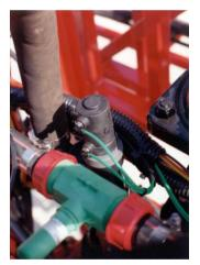
Situated at the rear of the tank on top of the manifold assembly, this valve is probably the most important item on the machine. It is pneumatically operated in two directions and controls the flow of water to the tank.
