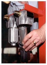
All return oil, except wheel motor drainage, passes through two 10  $\mu$  'Top Flow' filters - UC-2418 before re-entering the tank. Wheel motor drain oil returns to tank via an internal magnetic filter, and finally a 40  $\mu m$  strainer is fitted into the filler cap, primarily to filter air entering the reservoir and secondly to ensure clean oil only enters the reservoir.
