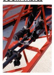
These valves are to an exclusive failsafe design. Air pressure at a minimum 7 bar (100 psi) is required to open the valves and so allow water to pass to the spray lines. When the air pressure is released, the valves, acting under very strong spring pressure, will close instantly. NB. See 'Main ON/OFF Valve'.
