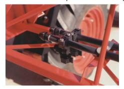
Fitted at 1/2 metre spacing along the spray lines are diaphragm check valves (DCV's). The valves eliminate dripping when the spray is turned off. If drips are present, it usually indicates dirt under the diaphragm. The spray tips fitted into the quick-fit bayonet caps usually of the ceramic type. These tips are very hard wearing and have a longer life expectancy than conventional tips.
