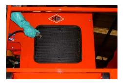
Particular attention should be paid to the hydraulic oil cooler sited on the far left-hand side of the cowling. Not only should it be cleaned thoroughly from inside the cowling but it should also be 'back blown' from the outside into the cowling. The removal of the small inspection plate to the left-hand side of the removable cowling will aid inspection.
