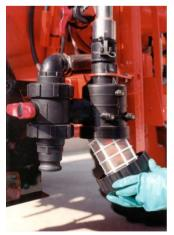
With the spraylines turned off and 'Tank Wash' selected the machine should be operated as for 'calibrating' the spraying system i.e. 9k/man 'ON' and main On/Off 'ON'. This will generate spray pressure and flush the water through an 'intank' cleaning nozzle. After 2-3 minutes of tank cleaning the 'tank wash' may be turned 'off' and the spraylines turned 'on'.
