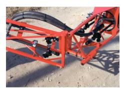
The boom can be used at these various widths but care should be taken, as the breakback section becomes inoperative when the end section is folded.
