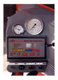
The control panel is mounted inside the cab in front of the pneumatic panel and houses all the controls necessary for operating the system.
