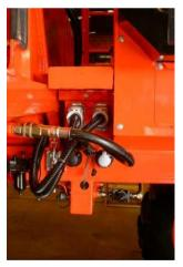
An unloader valve is mounted on the air tank inlet port. This is preset to maintain the air pressure at approximately 9 bar (130 psi). Absolute minimum working pressure is 7.5 bar (110 psi).
